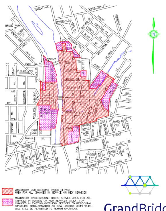
NOTE: ENERGY+ FEEDER CIRCUITS WILL BE OVERHEAD IN CORE AREAS.
